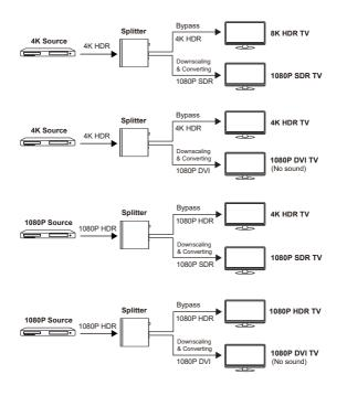
Note: If the source resolution is downscaled and converted to 1080P DVI according to the EDID of display devices, it will be output without sound on TV.
