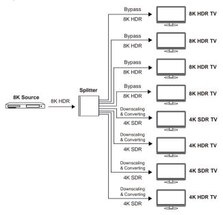
In the example above, 4K is lower than the resolution of input source, so it will downscale and output according to the the minimum resolution of 4K SDR.
