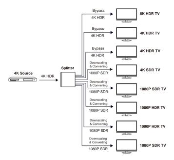
In the example above, 1080P is lower than the resolution of input source, so it will downscale and output according to the the minimum resolution of 1080P SDR.
